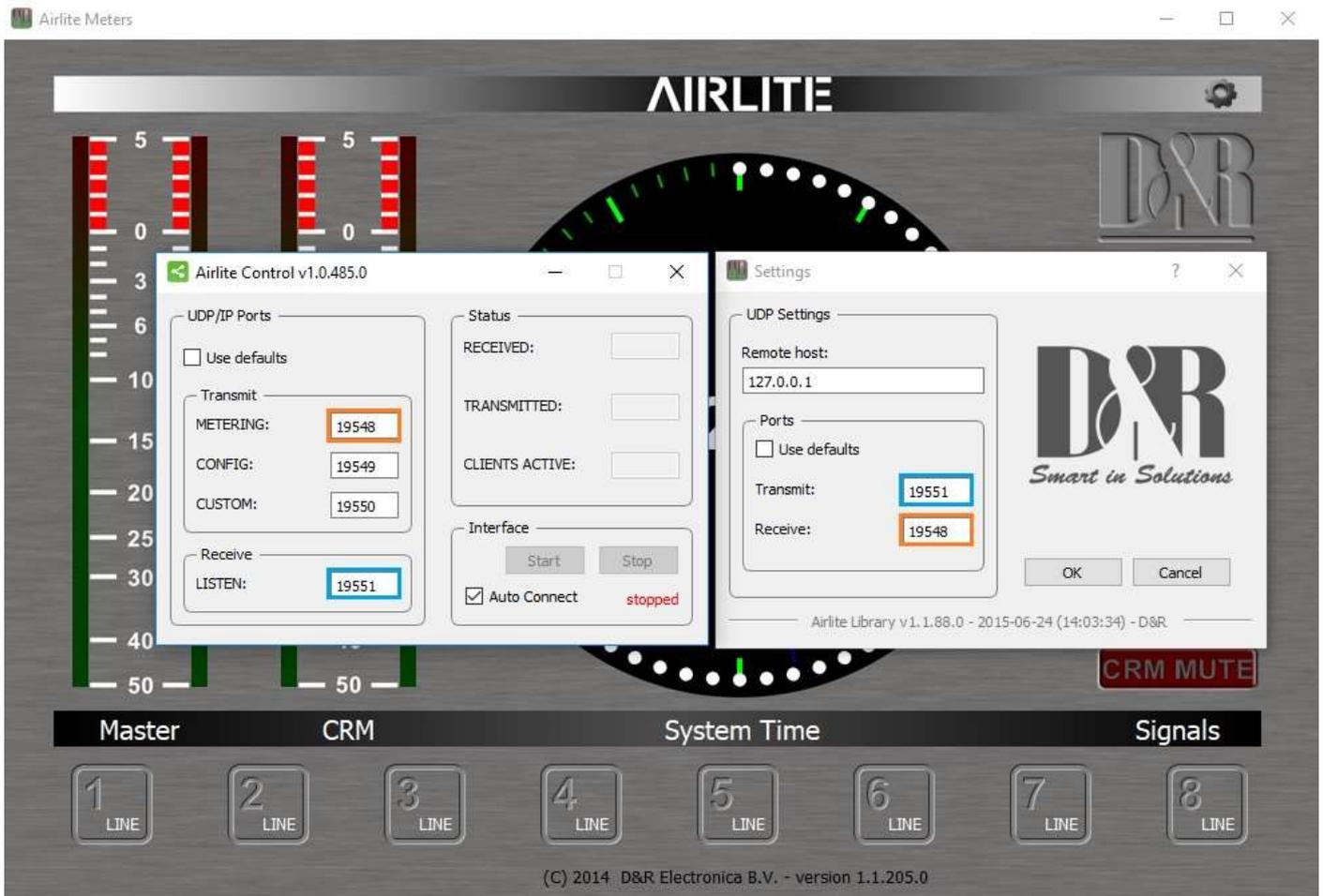
In blue you'll see the port that is used for transmitting the data to control the On switches with the software. (Software to Airlite).
