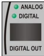
This section allows you to set up the digital output of the Sycos. The select button addresses the analog– or digital input as source for the digital output.
