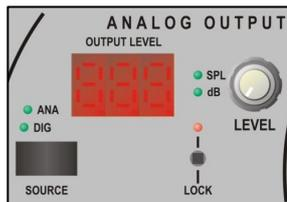
The analog output is operated in the same way as the digital outputs. The source select enables you to address either the digital- or analog input.
